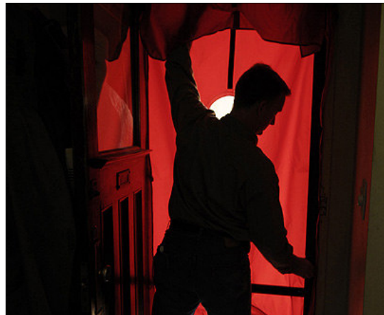
TONY BOCK/TORONTO STAR Don Noble, an inspector with Greensaver, does an energy audit on a reporter's house. He seals the front door to check the home's airtightness.
